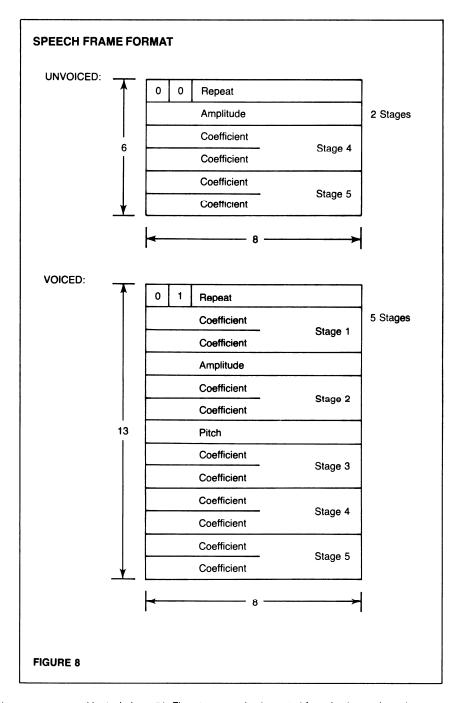
The speech data was compressed by technique #1. Five stages are implemented for voiced speech, and two stages for unvoiced speech. The driver routine is easy to implement, yet the ROM stores 30% more speech data than the non-compressed 15 x 8 bit format.
