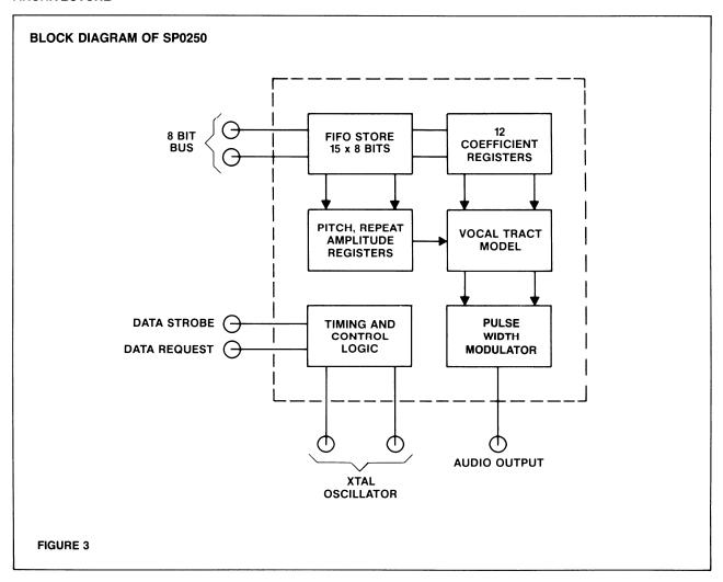
The SP0250 is controlled by 15 programmable eight bit parameter registers which hold the following information: voiced/unvoiced, pitch period, repeat count, amplitude and 12 digital filter coefficients (Figure 3).
