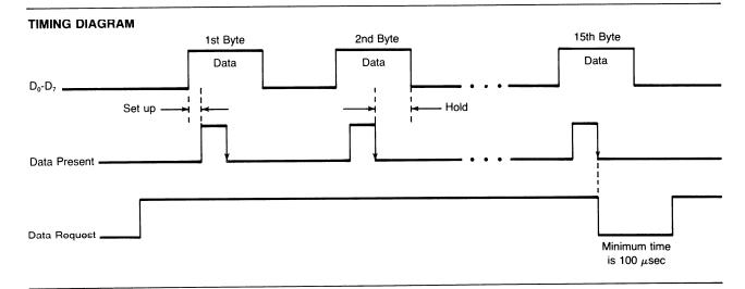
Data Request and Data Present are the handshaking signals used by the SP0250 and the microcomputer to transfer speech data. The SP0250 drives the Data Request line high when it is ready to accept a 15 x 8 bit speech frame (Data Request stays high until the entire frame has been input). When the microcomputer sees a logic 1 on
