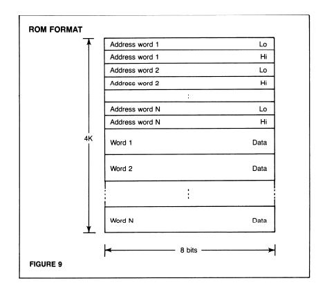
The ROM is divided into two sections — the jump table and the speech data. Each jump table entry points to the starting address of a particular segment of speech data. If there are ten words stored in ROM, then there will be ten two byte entries in the jump table. The speech data for each word will consist of compressed speech frames.
