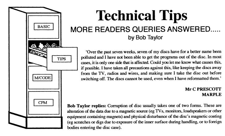
Physical disturbance causes the disc to be permanently faulty, while magnetism can have either temporary or permanent effects depending on the strength of the external magnetic field causing the corruption; a very strong field may magnetise the disc's magnetic material beyond the level which the disc drive head can alter.
