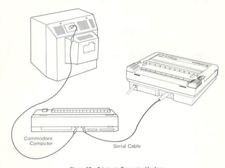
Figure 12. Printer to Computer Hookup
