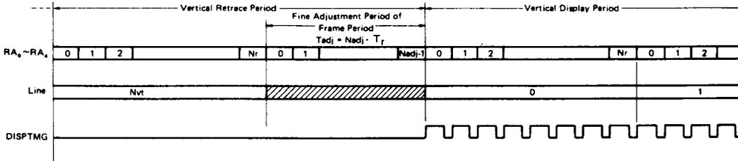
Figure 12 Fine Adjustment Period of Frame in Vertical Display
