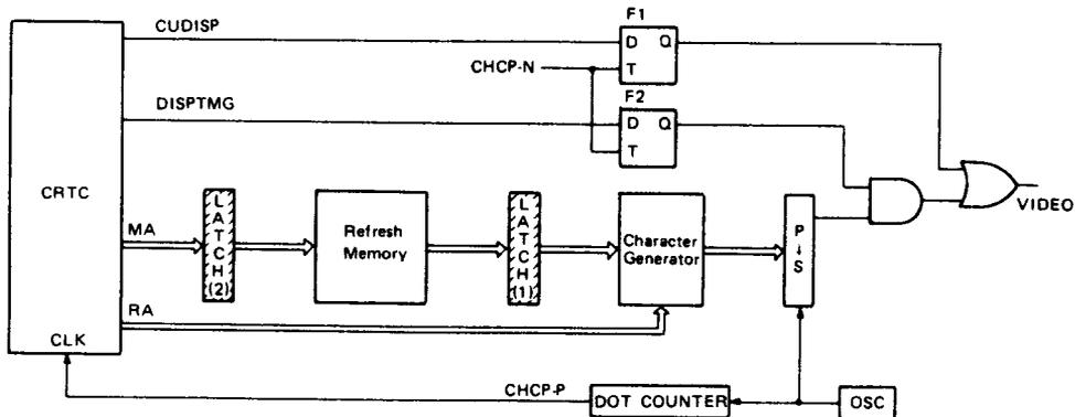
Figure 23 Display Control Unit (For high-speed display operation) (3)
