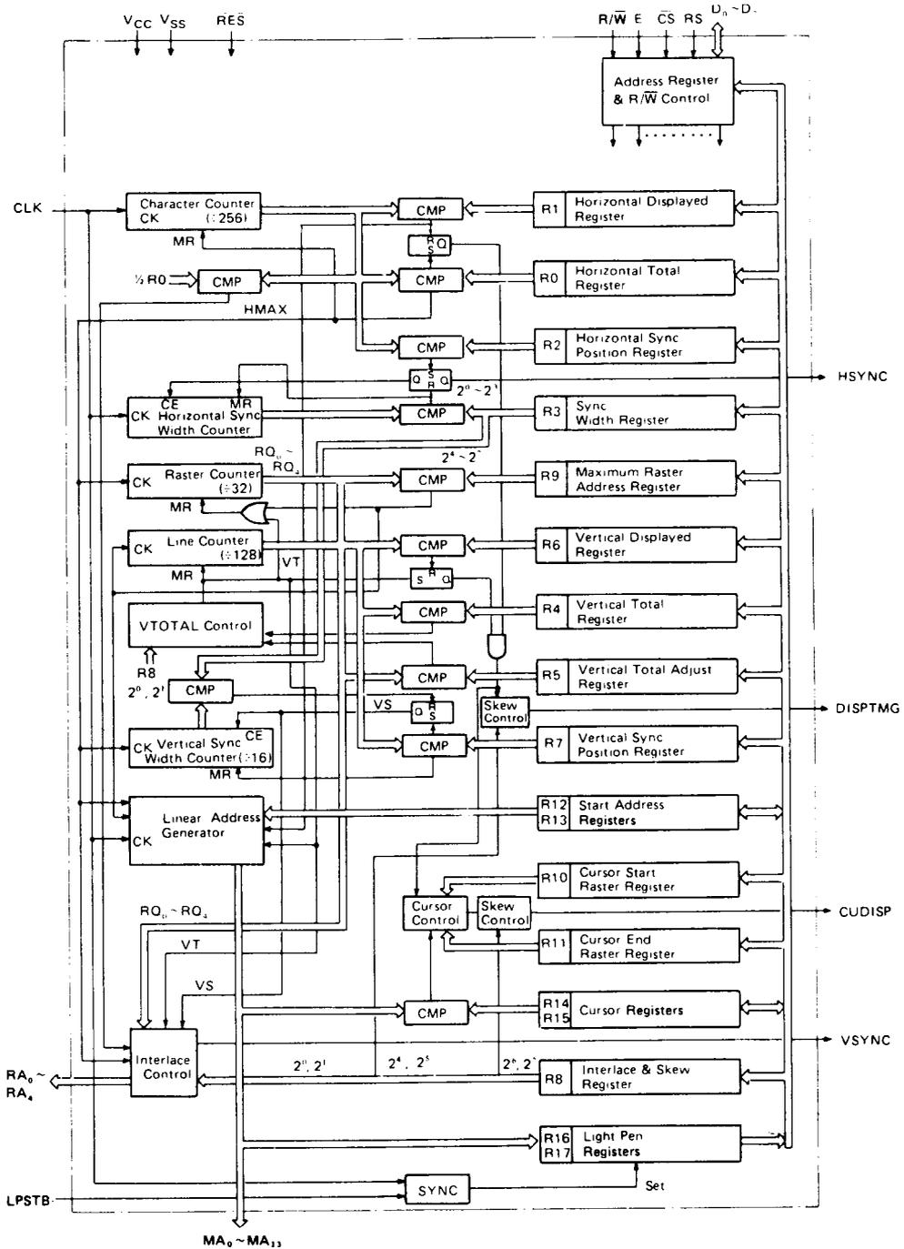
Figure 6 Internal Block Diagram of the CRTC
